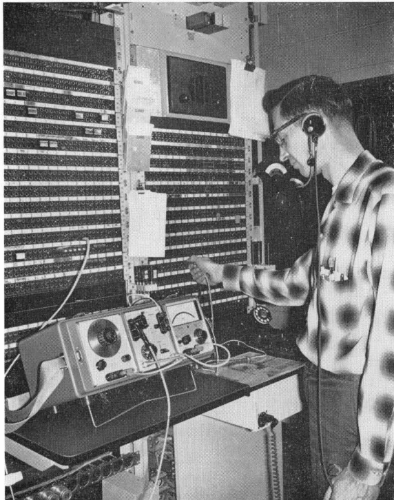
Fig. 1 (above). -hp- 3550A Portable Test Set with panel cover removed.
